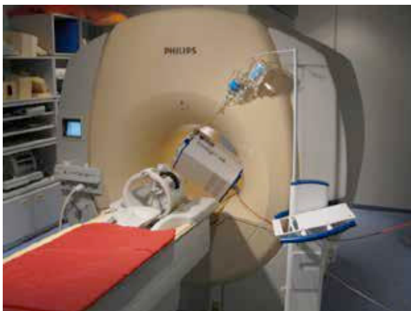
Figure 1.2: "MRI-compatible" contrast agent pump in a Philips Intera (1.5 T)
